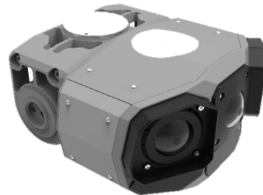
Figure 1. Proposed multi-sensor system. Each sensor module consists of a wide-angle camera, LiDAR, DGPS, IMU, embedded computer, and local area network.
