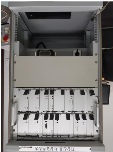
Fig. 4 On-board Measuring Equipment for Ground Signaling System
